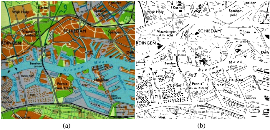
Fig. 3. Binarisation method of colour documents. (a) Original colour document, (b) Binarisation method based on a processing strategy involving two distance-based reduced orderings (dL) aiming at extracting black and dark blue characters.
